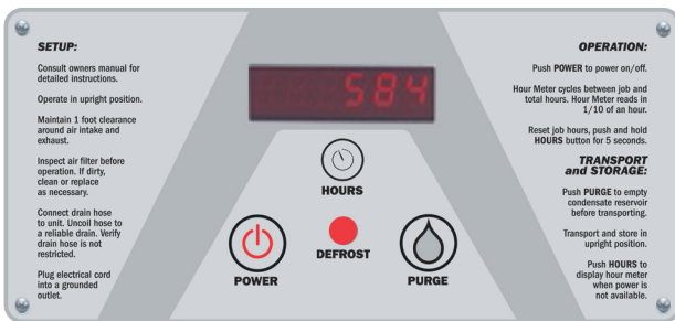
Figure 2: Phoenix R175 control board.
